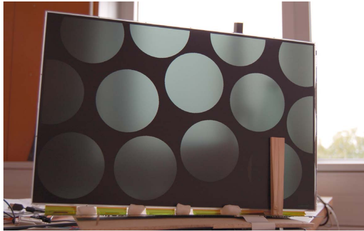
Figure 2.37: An LCD was disassembled to be used as a component for an HDR display. Here, white circles on a black background are displayed.
