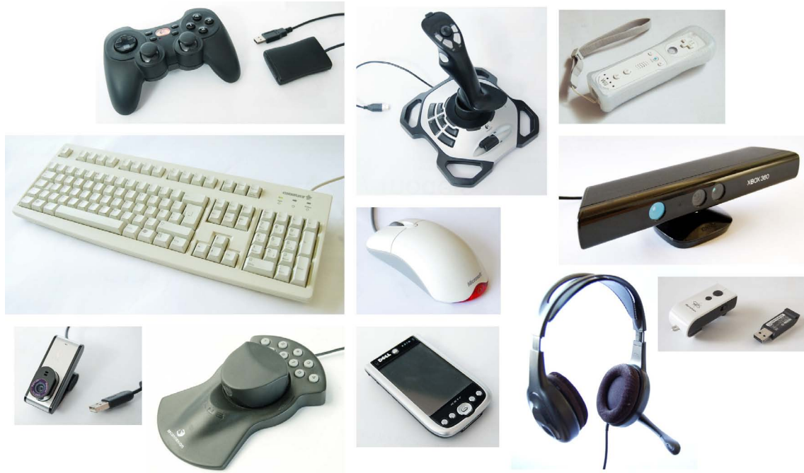
Figure 2.14: A selection of commercially available input devices. Depending on the setup, different devices make sense. Top row (left to right): wireless gamepad, joystick, wiimote. Center row: keyboard, mouse, kinect. Bottom row: webcam, spacemouse, PDA, headset, gyration mouse.
