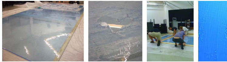
Figure 2.48: Silicone coating the large screen did not work well. The left two images show our first attempt that failed. Even using silicone thinner, our second attempt was not perfect, resulting in air bubbles and sometimes unregular spots as seen in the close up on the right.
