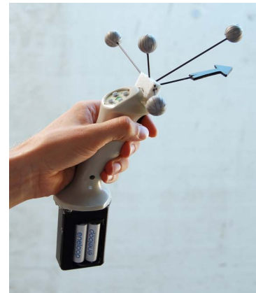
Figure 2.53: A custom joystick, a versatile input device used in most DAVE applications.
