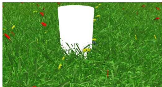
Figure 6.64: We ported the shader from Instant Animated Grass [HWJ07] to GLSL and adapted it to correctly work with instantreality in the DAVE. Similar to parallax mapping, the grass is rendered just a single quad, a ray casting is performed in the fragment shader, that even allows correct handling of depth, which is demonstrated here with the white cylinder. Horizontal and vertical slices of grass textures are used and slightly distorted over time to create a wind effect.
