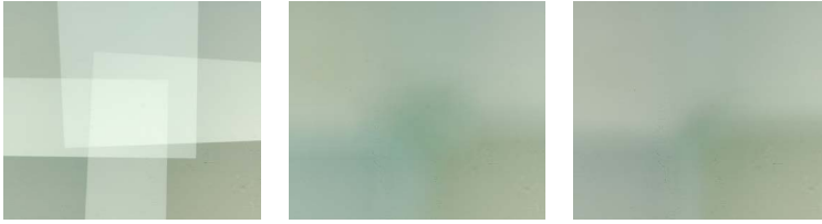
Figure 4.12: A close up view of a setup with only roughly mechanically aligned projectors. No blending, d^1 by Raskar et al. and d^4 with p = 1.5 (from left to right).
