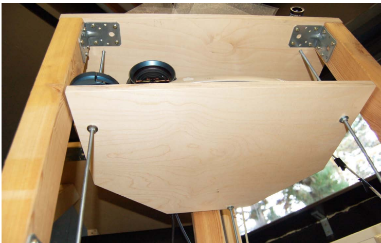
Figure 2.57: The custom stands allow an easy and precise adjustment of the projectors with three screws for each platform.
