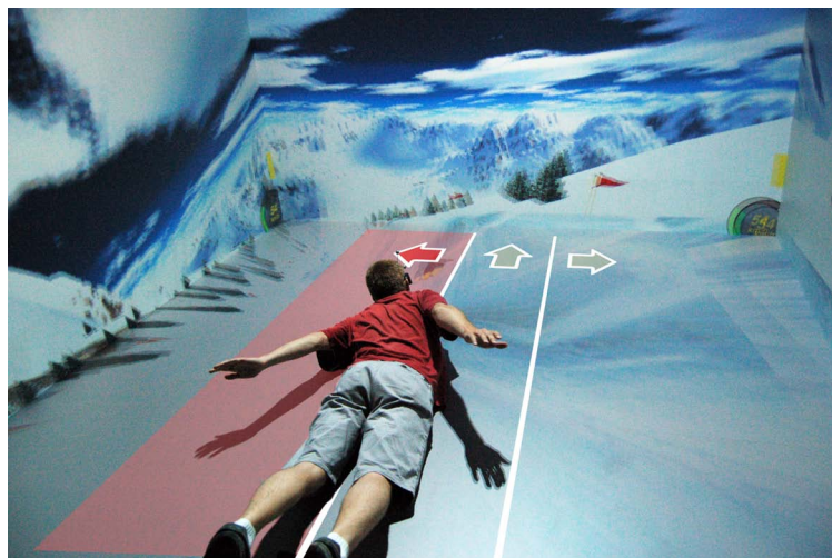
Figure 5.1: A simple control only using the absolute position of the glasses. Left, center and right positions are used for steering as indicated by arrows that are overlaid on the photo for illustrative purposes. When the glasses are higher than 1.4m above the ground, the penguin brakes. When they are lower than 0.8m above ground, the penguin speeds up.
