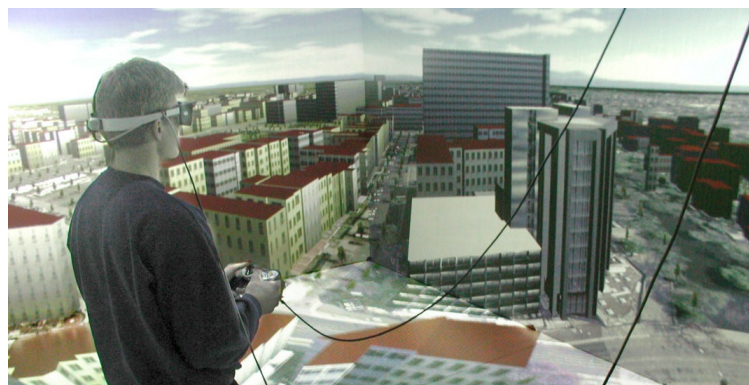
Figure 6.50: An automatically generated 3D city model of 200km 2 of Braunschweig in the first DAVE at TU Braunschweig. The data illustrated in the figure above served as input. The building on the right is one of the few detailed buildings that were modeled manually.
